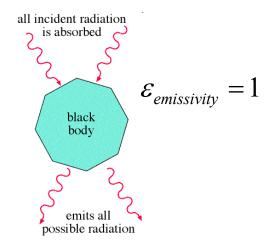
• Real object (ε<sub>emissivity</sub>)<1), replace T in (1) by
