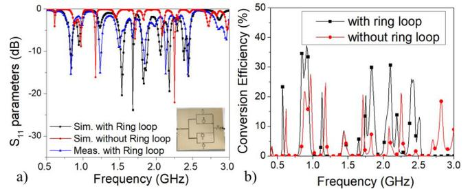
Fig. 4. (a) Reflection coefficient of the proposed multiband rectifier. (b) Conversion efficiency of the rectifier with and without ring loops.
