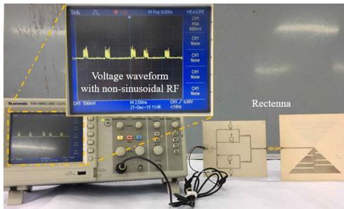
Fig. 6. Actual rectenna dc output voltage due to nonsinusoidal RF sources.
