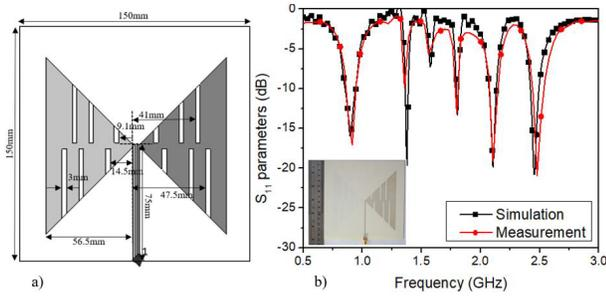
Fig. 2. (a) Proposed bow-tie antenna with its dimensions. (b) Comparison between simulation and measurement  $S_{11}$  parameters of the antenna. The inset illustrates the antenna fabrication.
