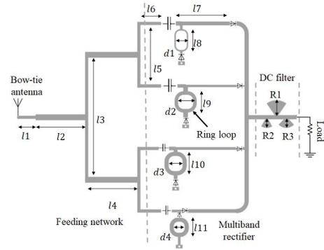
Fig. 3. Schematic of the multiband rectifier with ring loops.  $l_1 = 10$ ,  $l_2 = 24$ ,  $l_3 = 63$ ,  $l_4 = 23.5$ ,  $l_5 = 31.8$ ,  $l_6 = 10$ ,  $l_7 = 27.6$ ,  $l_8 = 9$ ,  $l_9 = 6.5$ ,  $l_{10} = 7$ ,  $l_{11} = 5$ ,  $d_1 = 5$ ,  $d_2 = 7$ ,  $d_3 = 6.5$ ,  $d_4 = 5$ ,  $R_1 = 8$ ,  $R_2 = 4$ ,  $R_3 = 4$ , all units in mm.
