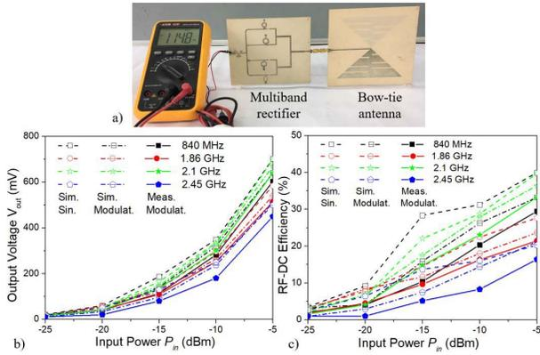
Fig. 5. (a) Rectenna measurement in ambient with a voltage meter. (b) Simulation and measurement output voltage results. (c) RF-dc efficiency of multiband rectenna at four desired frequency bands.
