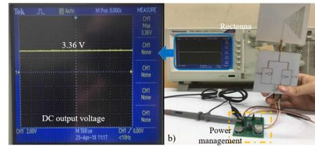
Fig. 7. (a) Block diagram of the power management. (b) Measurement of the rectenna with power management circuit.
