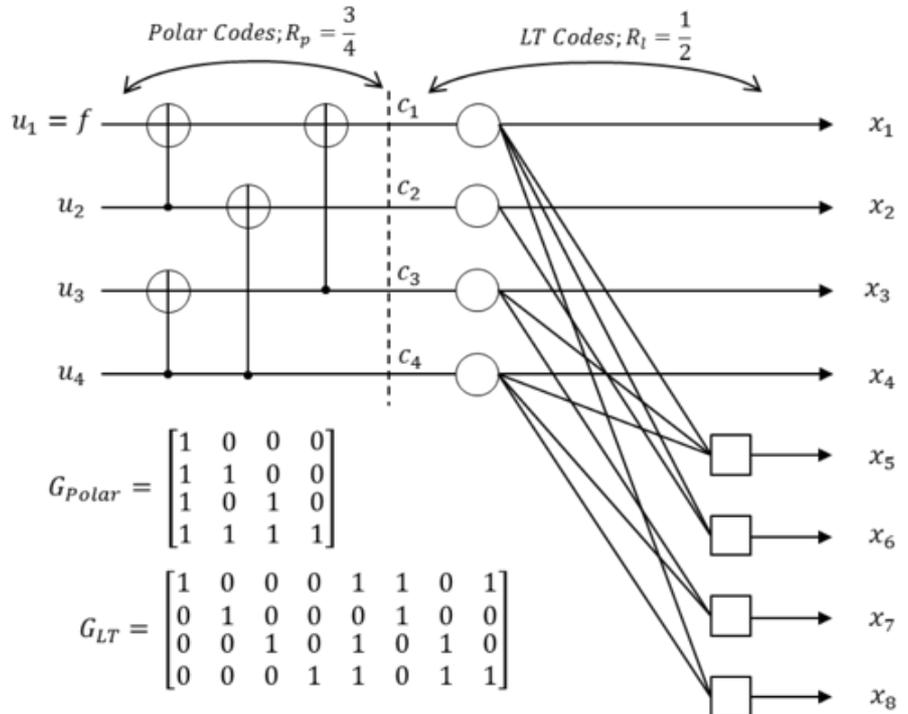
Figure 2. Construction of Polar-LT Codes, in the transmitter side.
