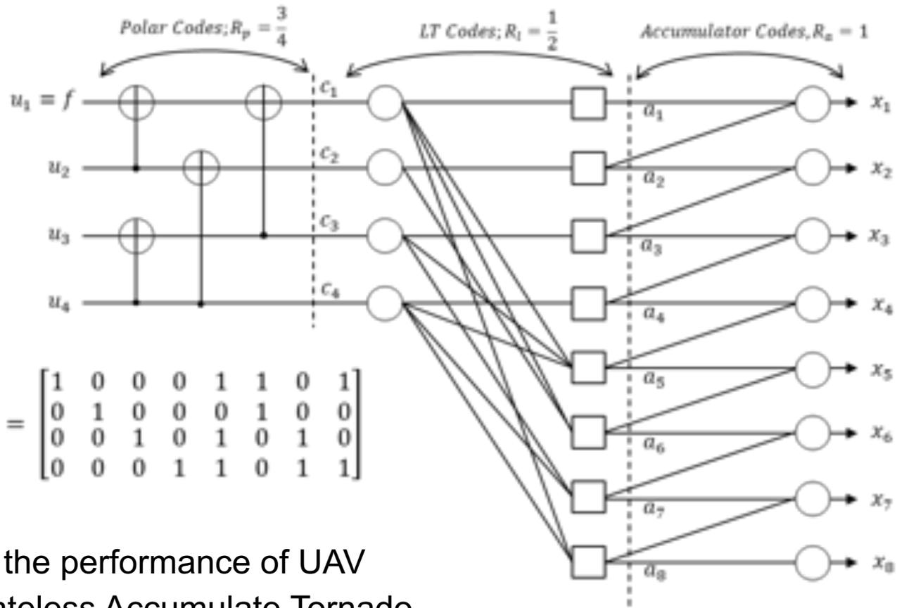
Figure 2. Construction of Rateless Accumulate Tornado Codes, in the transmitter side.
