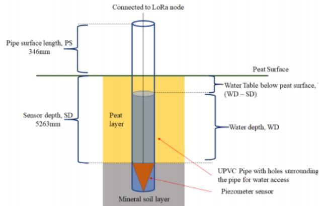
Fig. 3. Piezometer installation layout.
