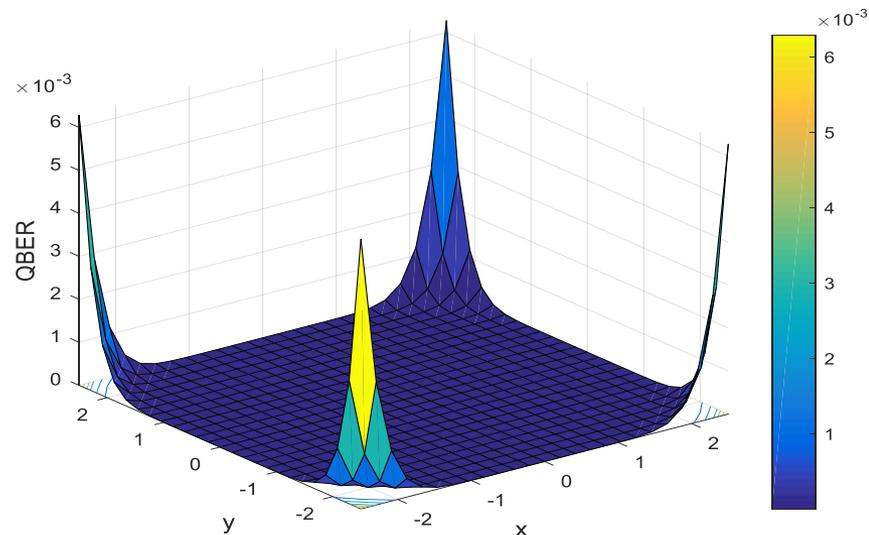
QBER versus different Bob's locations when the dual-threshold scale coefficient  $\delta = 1.5$ , the intensity modulation depth  $\rho = 0.25$  and  $P_{LED} = -3$  dBm
