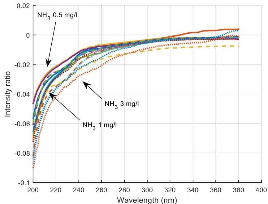
Absorption characteristics of  $\text{NH}_3$  from 0.05 mg/l to 3 mg/l
