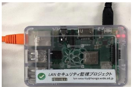
Fig. 2: Monitoring node of LAN-security monitoring project
