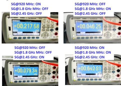
Figure 20. Measured output DC voltage according to different states of RF signal generators.
