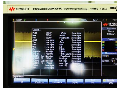
Figure 22. Detailed information of the measured output voltage waveform shown in Fig. 21.
