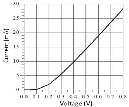
I-V characteristic of the SMS7630 diode
