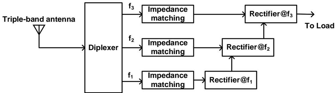
Figure 1. Schematic diagram of the proposed RFEH circuit.
