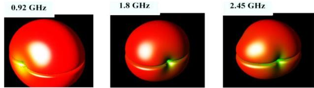
Simulated radiation pattern of the triple-band antenna.
