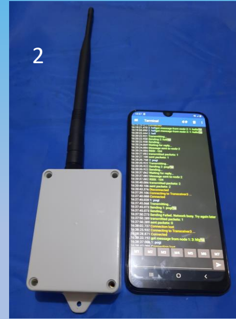
SMS-style communication using BLE and Bluetooth Terminal as interface
