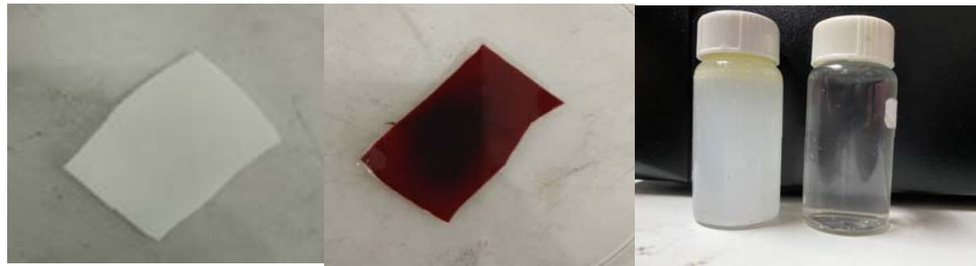
Fig. 1 PVDF membrane before and after lignin coating for removing oil emulsion (from left to right).
