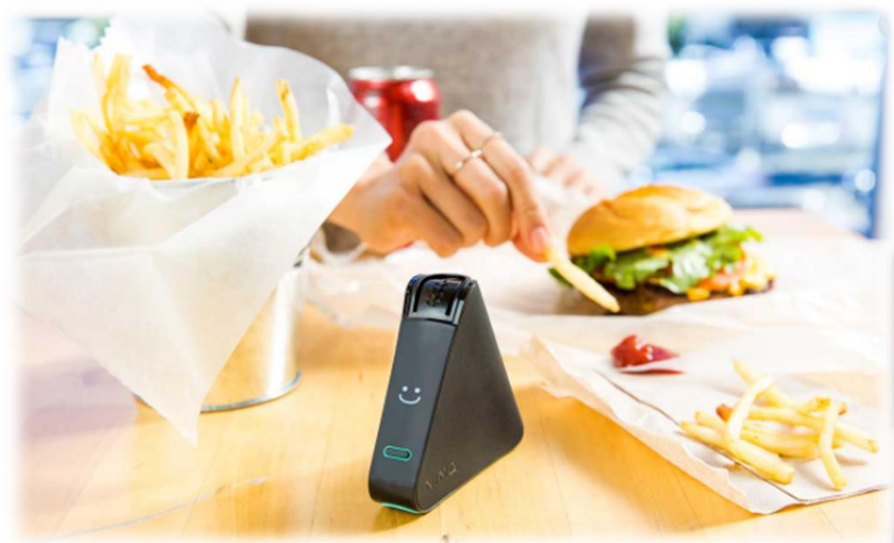
Nima: A portable sensor allows consumers to test food for gluten.
