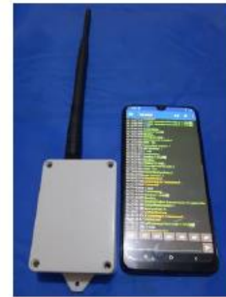
Node prototype of the LoRa-based Mesh Network
