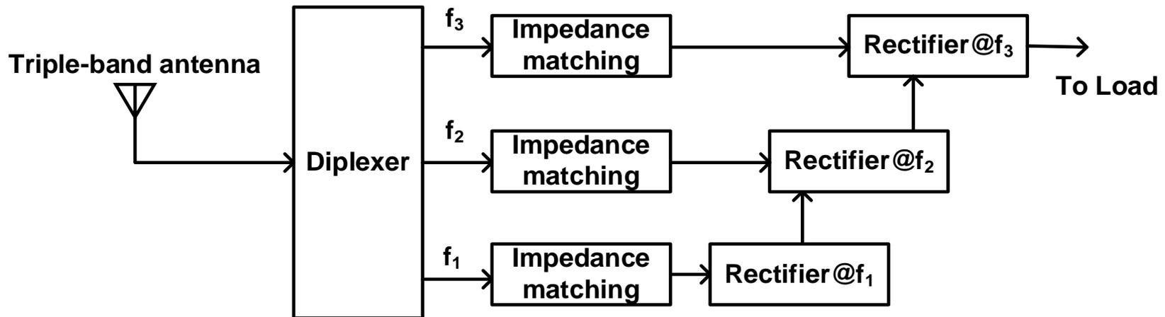
Schematic diagram of the proposed RFEH circuit.
