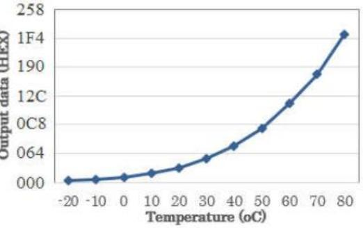
Digital Sensor Output vs. temperature
