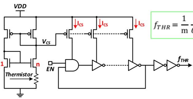
Fig. 2. Schematic of the temperature sensing element
