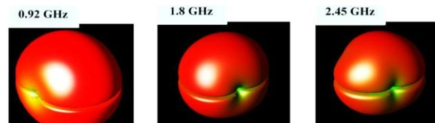
Simulated radiation pattern of the triple-band antenna.
