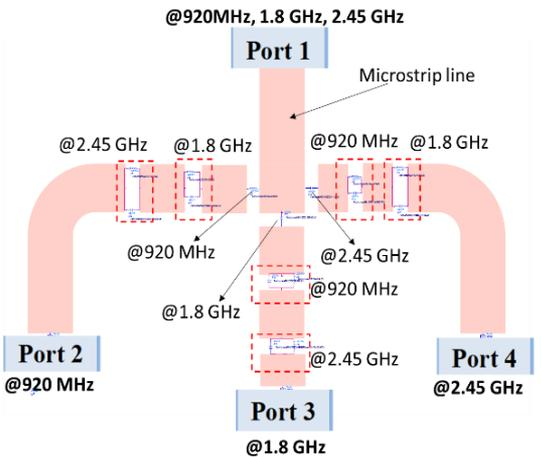
Co-simulation model for the designed diplexer. Total size of this circuit is 1.8 cm × 2 cm
