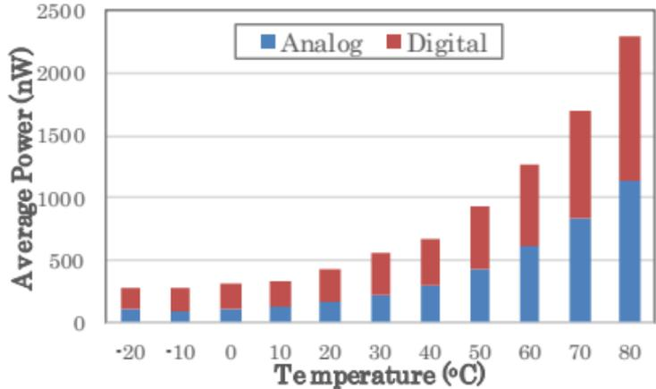
Fig. 8. The power average with the changing of temperature.
