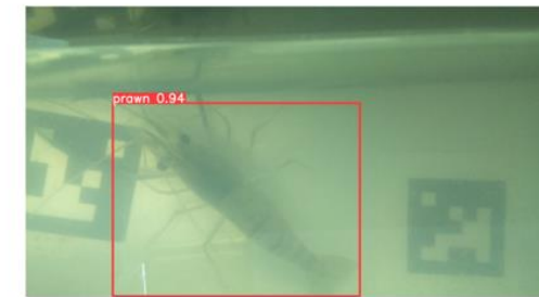
Fig. 4. High turbidity underwater freshwater prawn detection result using YOLOv8, with a confidence score of 94%
