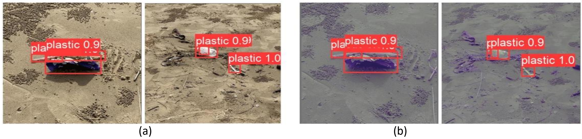
Figure 1: The detection of plastic waste samples by YOLOv5m model for (a) RGB images and (b) RGNIR images
