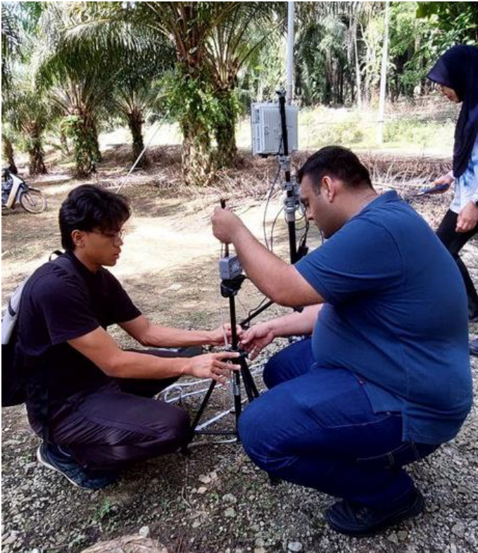
Measurement in the palm plantation using LOS and NLOS configurations (April-July 2024)
