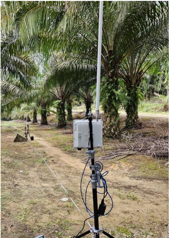
Measurement in the palm plantation using LOS and NLOS configurations (April-July 2024)
