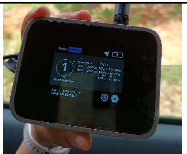
Measurement using 3 different end nodes (EN), including a proprietary (RAK Wireless) field tester
