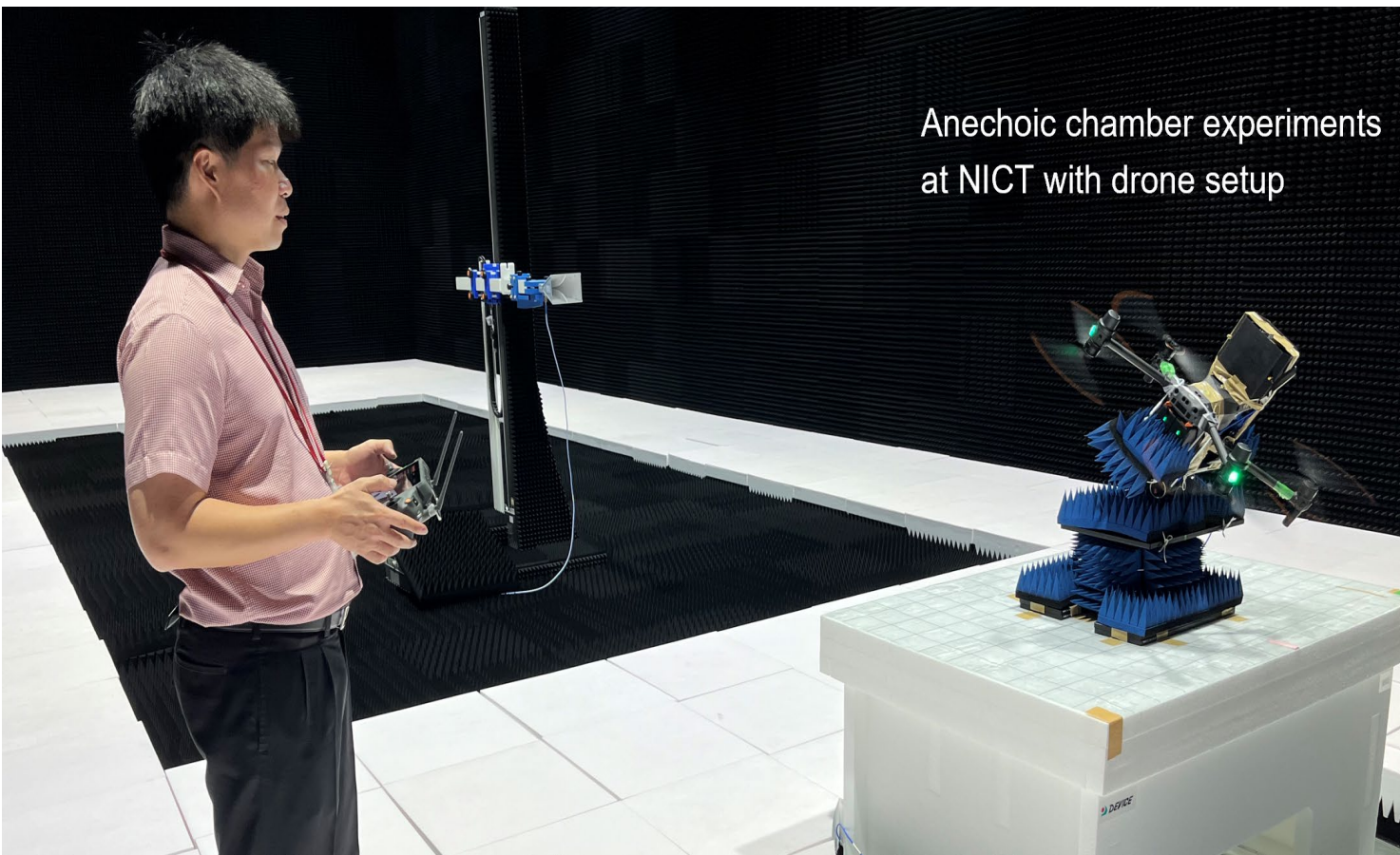
UAV setup tested in Anechoic Chamber to check for signal interference to ensure reliable connectivity to ground sensors.
