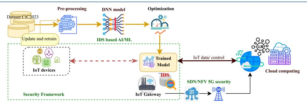
Security framework for agricultural IoT on Edge computing: IoT devices/networks security; SDN/NFV 5G connected networks; IDS based on AI/MLs.
