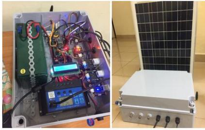
**Figure2. Designed of solar-based water-proof panel box**
